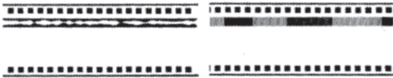
Left – variable area, width of transparent part varies with audio
